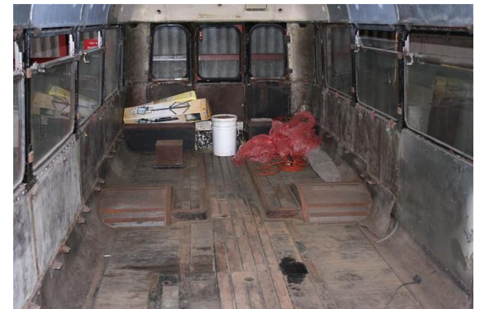
Restoration included removal of the wheelchair access door cut into the side; here the interior begins to recover its original form. Photo Colin Grafham collection
